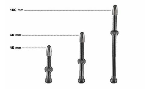
Schwalbe's new tubeless valves: The correct stem length and technical details – wider foot, shorter cone, Allen key socket, enlarged O-ring - facilitate handling and assembly.
